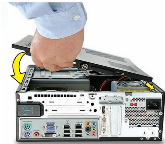
10 Tighten the side panel thumbscrew on the back of the computer.
