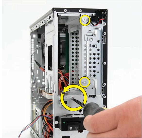
**17** Remove the screw at the top of the drive cage. (This is one of the short screws on select models.)
