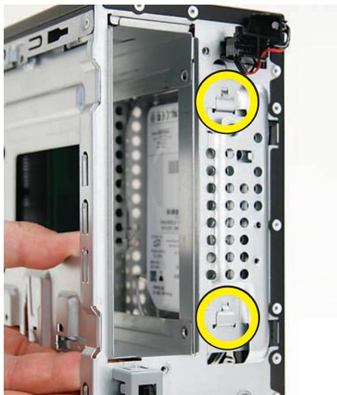
...ensure the screw hole at the top of the drive cage aligns under the screw hole in the computer rail (1).
