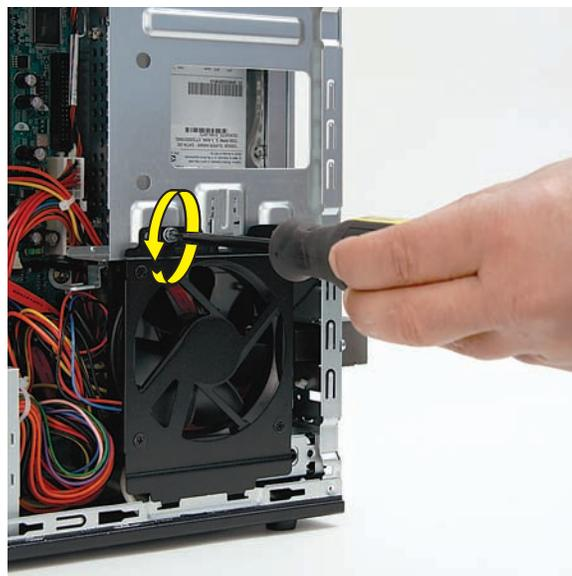
**16** Push in the metal tab (1) above the fan as you tip out the top of the fan (2), and lift the fan (3) partway out of the computer. Without disconnecting the fan, set it aside.
