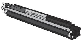
2. If the print cartridge does not appear to be damaged, rock the print cartridge gently several times and reinstall it. Print a few pages to see if the problem is resolved.
