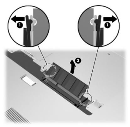
To protect the memory module after removal, place it in an electrostatic-safe container.
