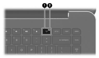
If the wireless light is amber, all wireless devices are off. If the wireless light is off, all wireless devices are on.
