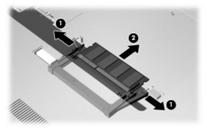
To protect the memory module after removal, place it in an electrostatic-safe container.
