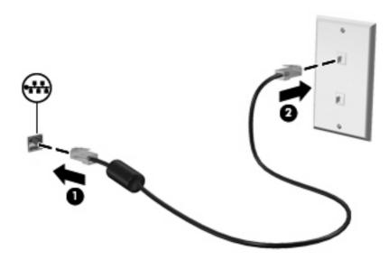
△ WARNING! To reduce the risk of electric shock, fire, or damage to the equipment, do not plug a modem cable or telephone cable into an RJ-45 (network) jack.
