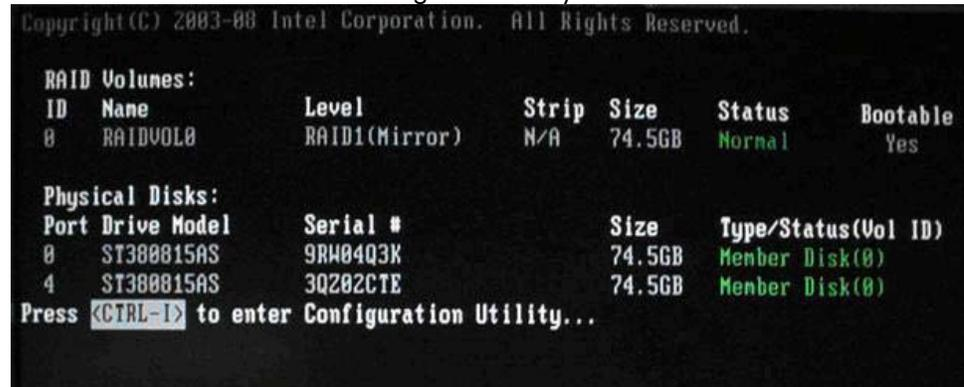
2. Press **Ctrl + I** repeatedly as soon as the monitor light turns green to enter the RAID configuration utility. If you do not press **Ctrl + I** at the appropriate time, you must restart the computer, and then press **Ctrl + I** again to access the utility.
