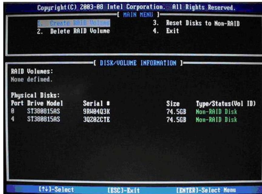
1. Use the up or down arrow key to select **Create RAID Volume**, and then press **Enter** to access the Create Volume screen.
