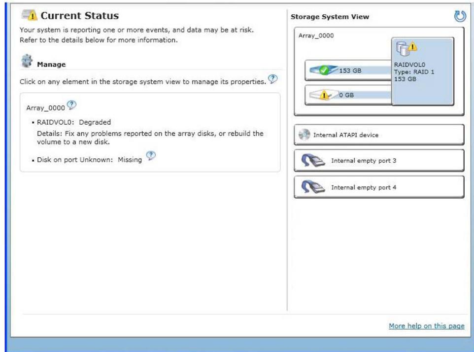
2. After identifying the hard drive, close all applications, shut down the operating system, power down the unit, unplug the power cord, and replace the defective hard drive.
