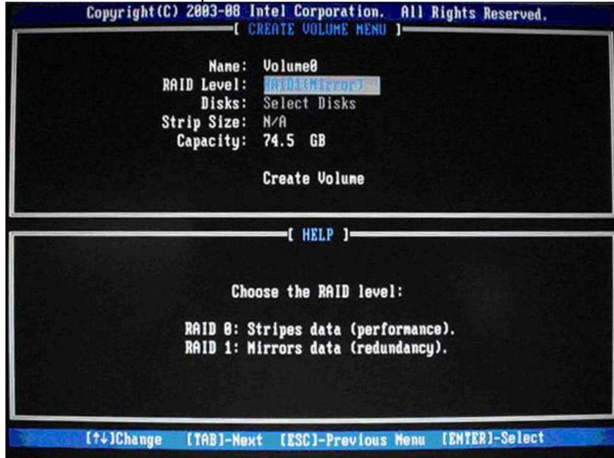
3. Use the arrow keys to scroll to **Create Volume**, and press **Enter**. The following screen appears. **WARNING: All data on the selected disk will be deleted.**
