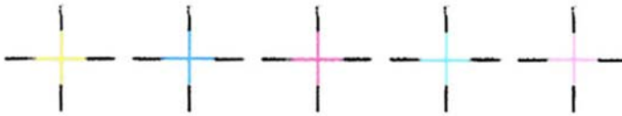
SCAN AXIS AND PAPER AXIS PRINthead REGISTRATION (DIE 1)
