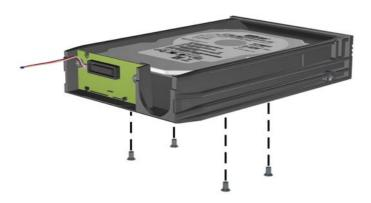
5. Slide the hard drive back to disconnect it from the carrier then lift it up and out of the carrier.
