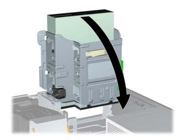
10. Press down on the green drive retainer button located on the left side of the drive to disengage the drive from the drive cage (1). While pressing the drive retainer button, slide the drive back until it stops, then lift it up and out of the drive cage (2).
