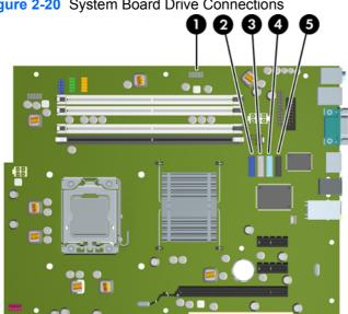
Figure 2-20 System Board Drive Connections
