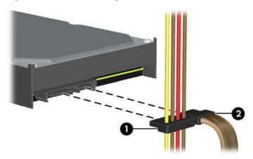
10. Press down on the green release latch next to the hard drive (1). While holding the latch down, slide the drive forward until it stops, then lift the drive up and out of the bay (2).
