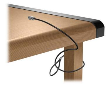
2. Thread the keyboard and mouse cables through the lock.
