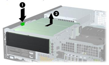
NOTE: To replace the drive, reverse the removal procedure. When replacing a drive, transfer the four guide screws from the old drive to the new one.
