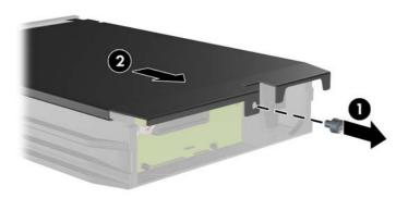
3. Remove the adhesive strip that secures the thermal sensor to the top of the hard drive (1) and move the thermal sensor away from the carrier (2).
