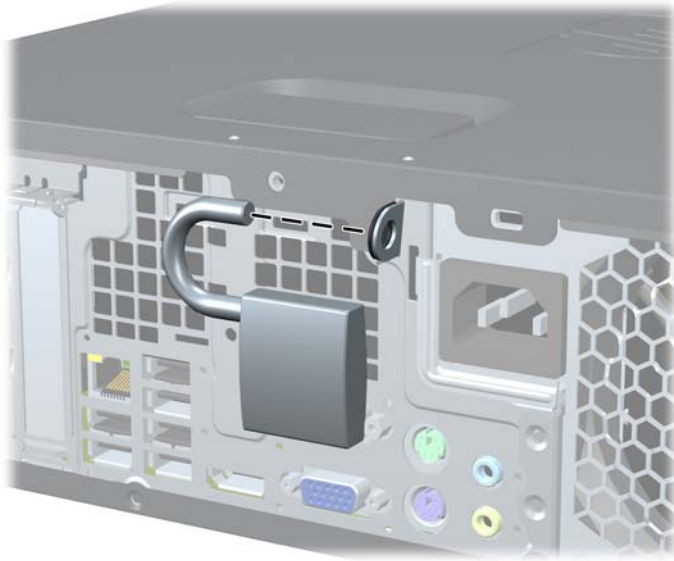
Figure C-2 Installation d'un cadenas
