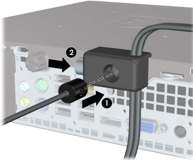
Figure C-7 Engaging the Lock
