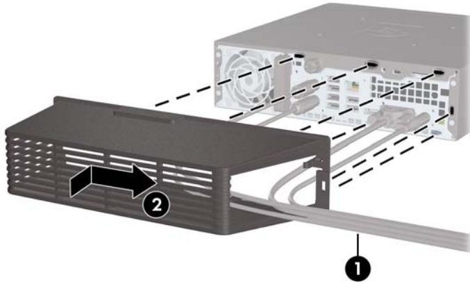
Figure 2-21 Installing a Port Cover
