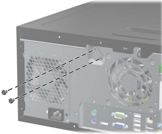
Figure 1 Removing the Smart Cover Lock Screws
