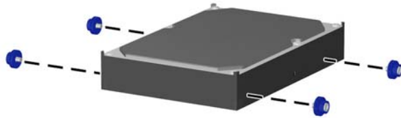
Figure 23 Installing the Hard Drive Guide Screws
