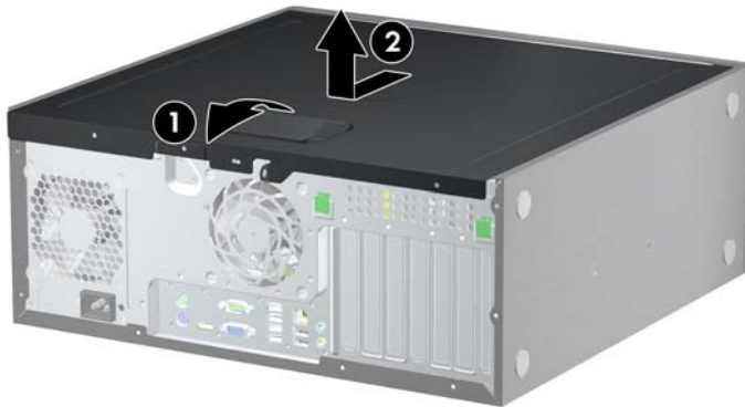
Figure 2 Removing the Computer Access Panel
