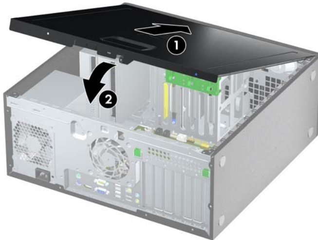
Figure 3 Replacing the Computer Access Panel
