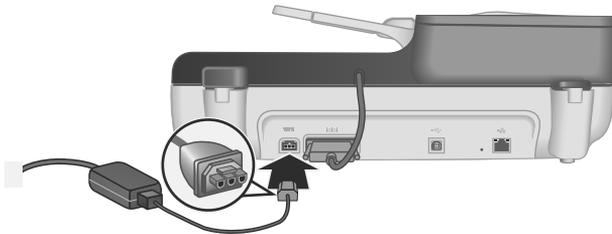
2. Plug the small end of the AC cable into the back of the power supply.
