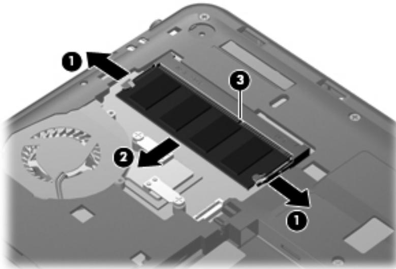
Reverse this procedure to install the memory module.
