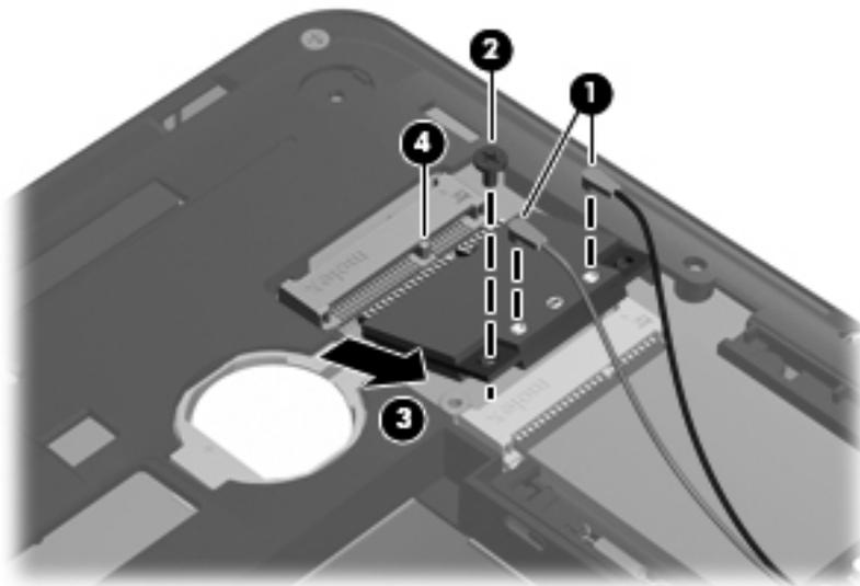
Reverse this procedure to install the WLAN module.
