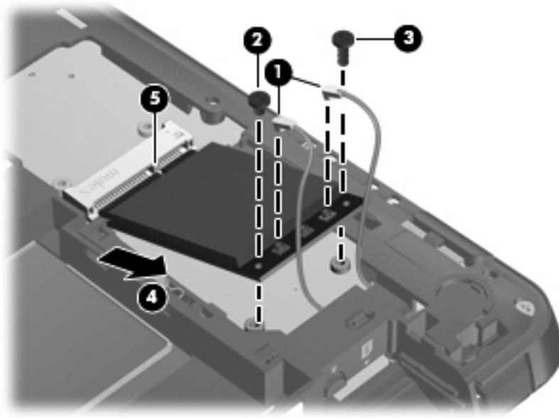
Reverse this procedure to install the WWAN module.
