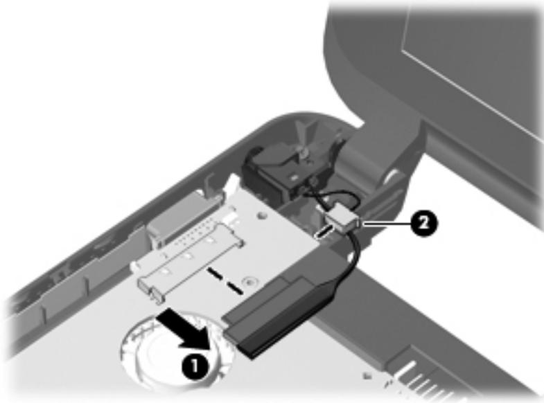
3. Remove the Phillips PM2.0×4.0 screw **(1)** that secures the system board to the base enclosure.
