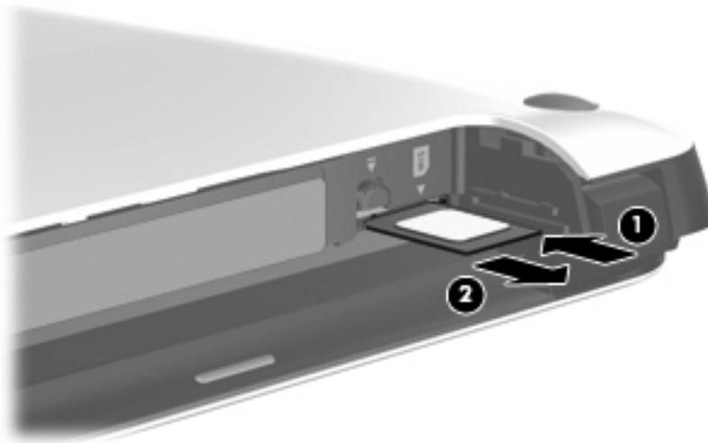
Install the SIM by inserting it into the SIM slot until you hear a click.
