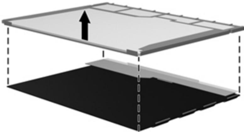
24. Recycle the LCD panel and backlight.
