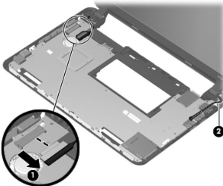
△ **CAUTION:** Support the display assembly when removing the following screws. Failure to support the display assembly can result in damage to the display assembly and other device components.
