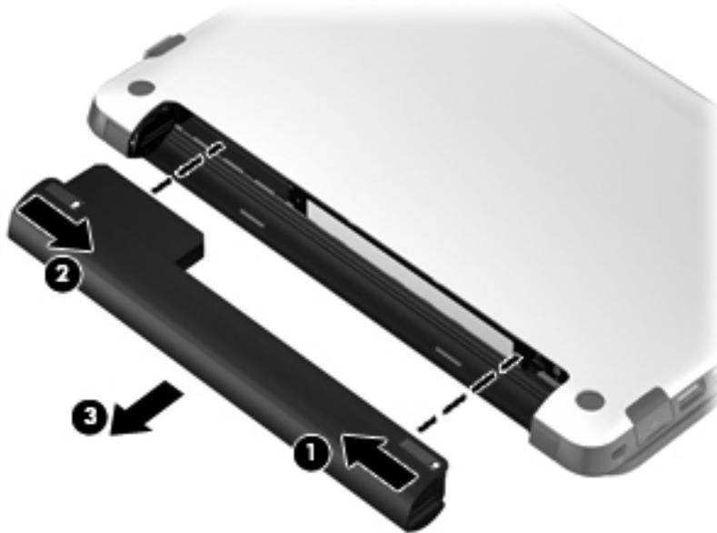
Reverse this procedure to install a battery.
