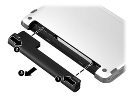
Reverse this procedure to install a battery.
