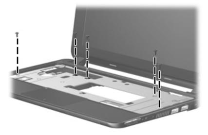
Release the top cover (1) by lifting the rear edge until it disengages from the base enclosure.
