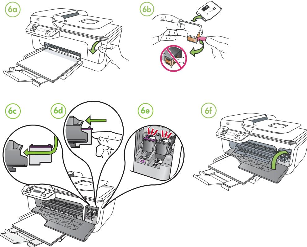
**(EN) Align the cartridges**
