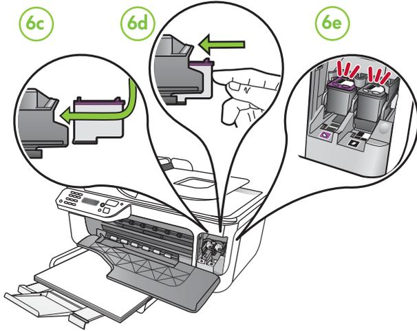
**EN** Align the cartridges
