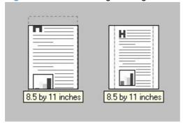
When the size for which the document is formatted (that is, the logical size) differs from the target size, the preview image uses a dashed gray line to show the boundaries of the logical page in relation to the target paper size.
