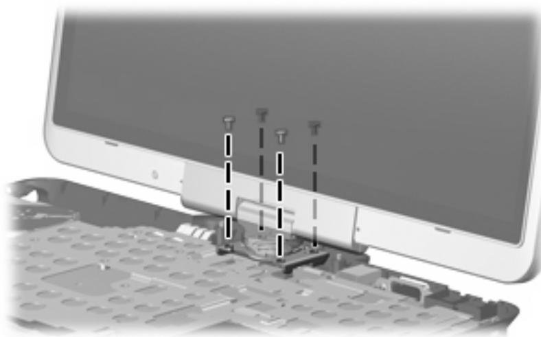
**Where used:** 4 screws that secure the display assembly to the base enclosure
