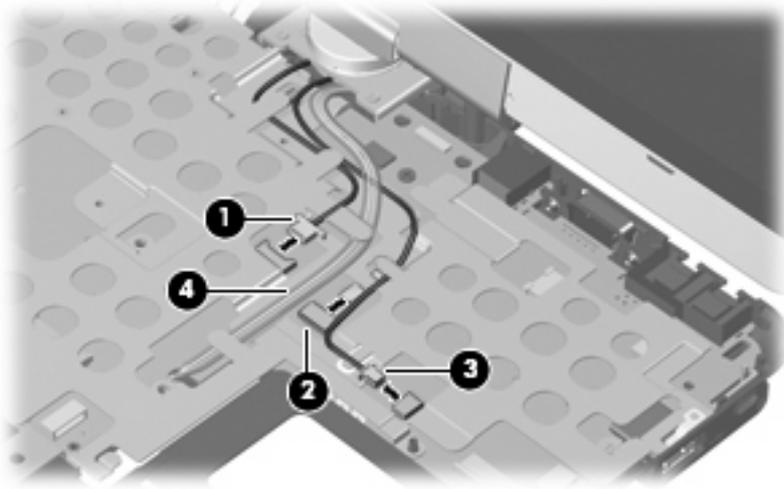
4. Remove the two Phillips PM2.0×6.0 screws (1) that secure the display panel cable to the system board.
