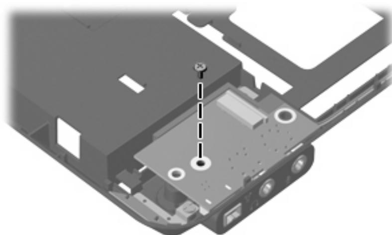
**Where used:** One screw that secures the audio connector board to the base enclosure
