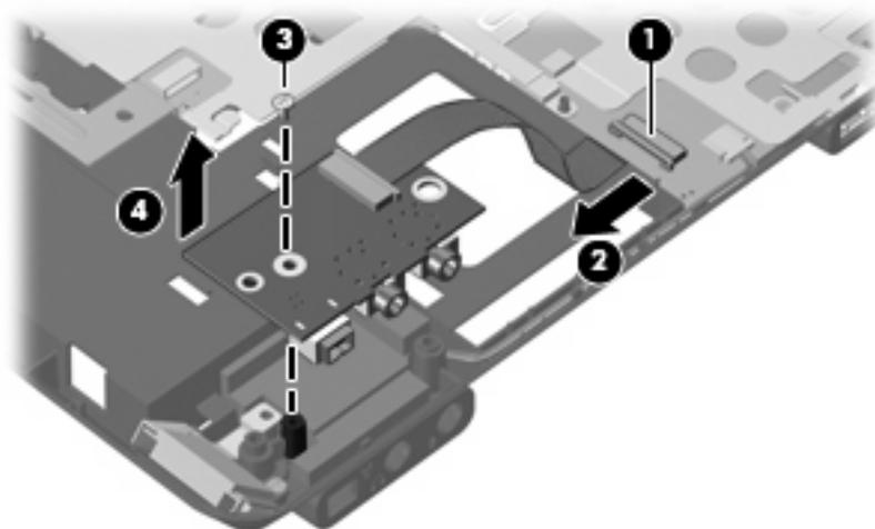
Reverse this procedure to install the audio connector board.
