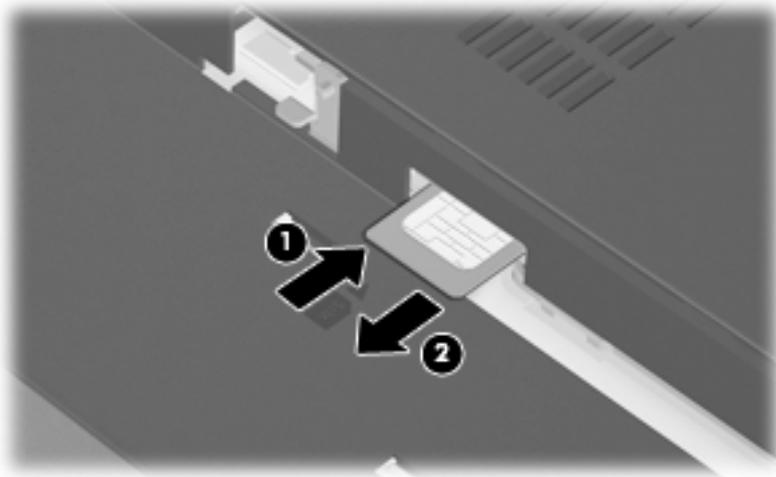
Reverse this procedure to install the SIM.
