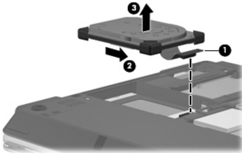
Reverse this procedure to install the hard drive.
