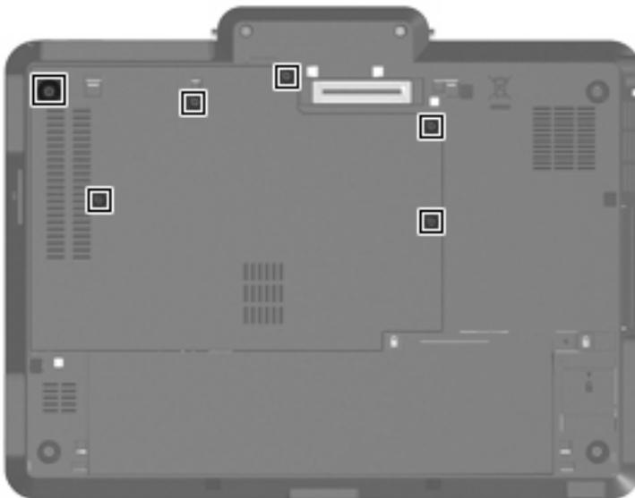
**Where used:** 6 captive screws that secure the hard drive compartment cover to the computer (screws are captured on the cover by C-clips)
