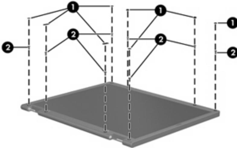
2. Lift up and out on the left and right inside edges (1) and the top and bottom inside edges (2) of the display bezel until the bezel disengages from the display assembly.
