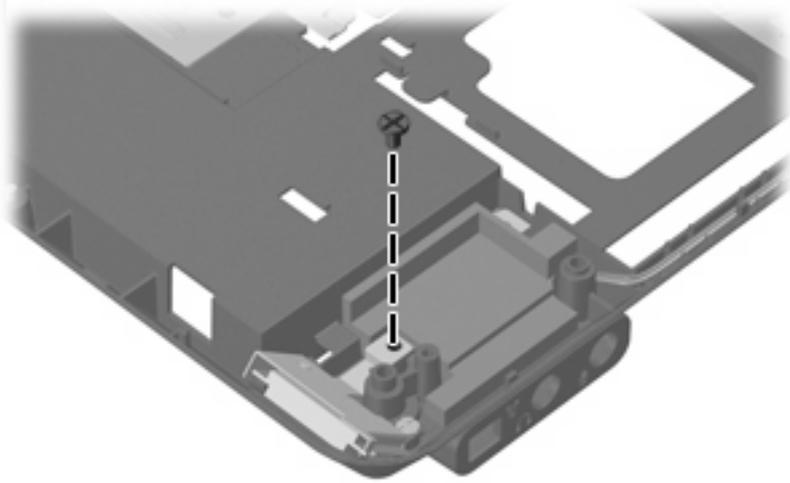
**Where used:** One screw that secures the Bluetooth module to the base enclosure
