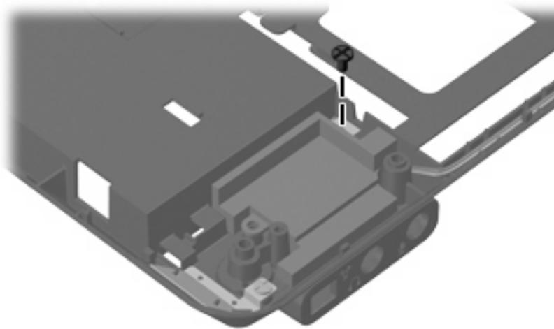
**Where used:** One screw that secures the speaker to the base enclosure
