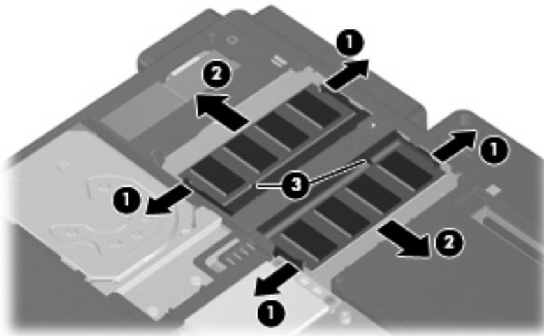
Reverse this procedure to install the memory module.
