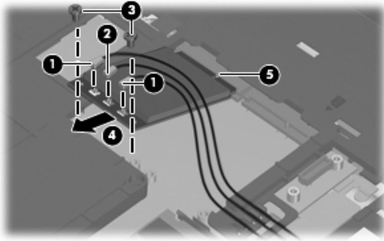
Reverse this procedure to install the WLAN module.
