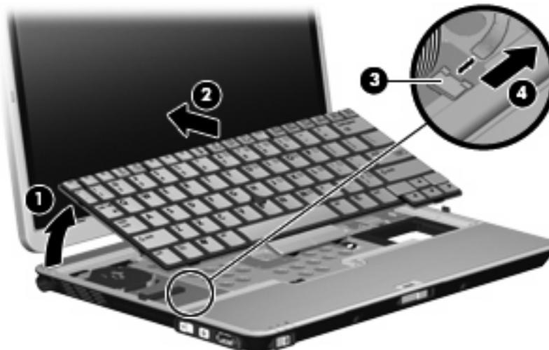
6. Swing the top edge of the keyboard (1) up and forward until it rests upside down on the palm rest.
