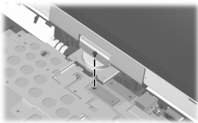
**Where used:** One screw that secures the display converter cable to the system board
