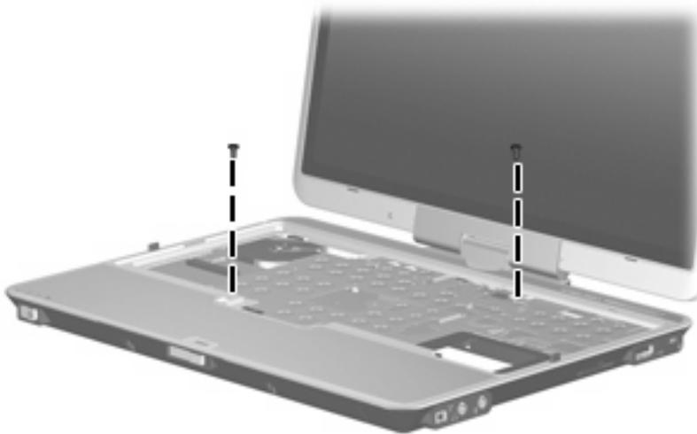
**Where used:** 2 screws that secure the top cover to the base enclosure
