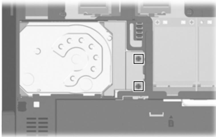
**Where used:** 2 screws that secure the hard drive bracket to the system board
