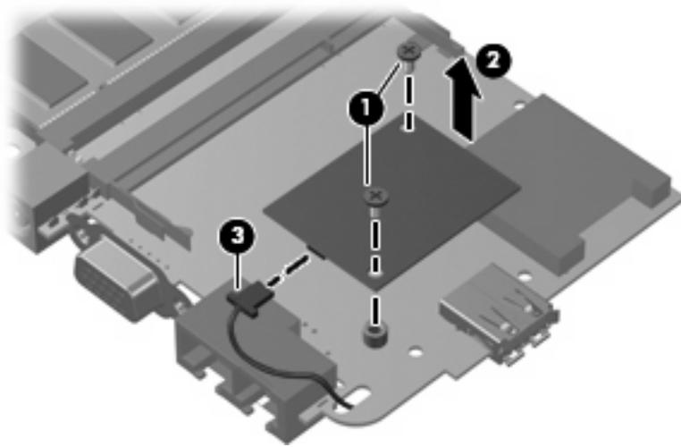
Reverse this procedure to install the modem module.
