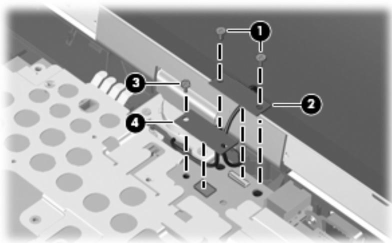
△ **CAUTION:** The display assembly will be unsupported when the following screws are removed. To prevent damage to the display assembly, support it before removing the screws.
