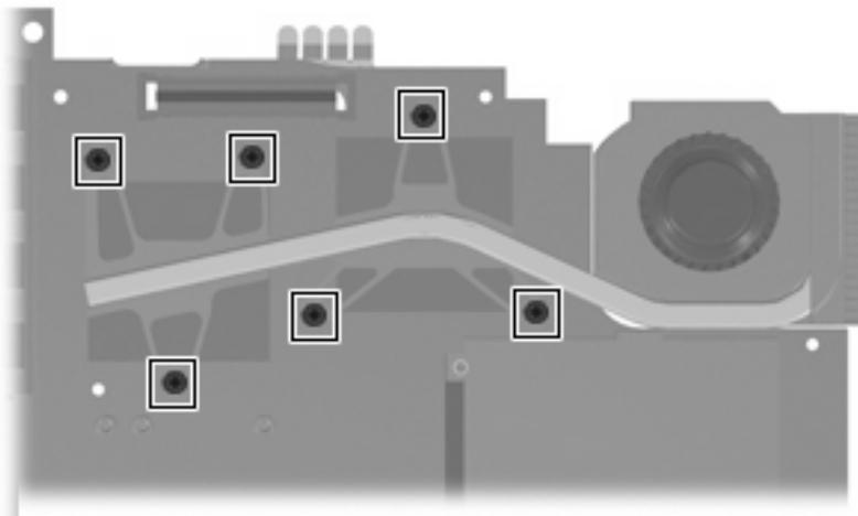
**Where used:** 6 captive screws that secure the fan/heat sink assembly to the system board (screws are captured on the fan/heat sink assembly by C-clips)
