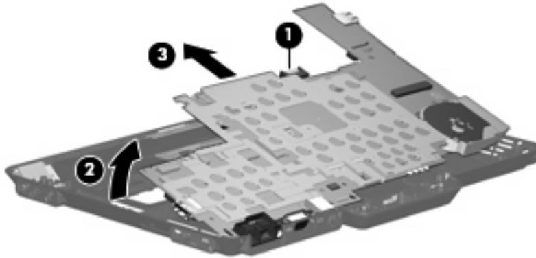
You can replace the heat shield that sits atop the system board using spare part number 458406-001.
