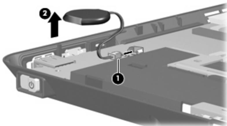
Reverse this procedure to install the RTC battery.
