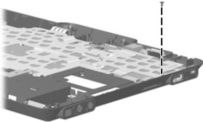
**Where used:** One screw that secures the system board to the base enclosure
