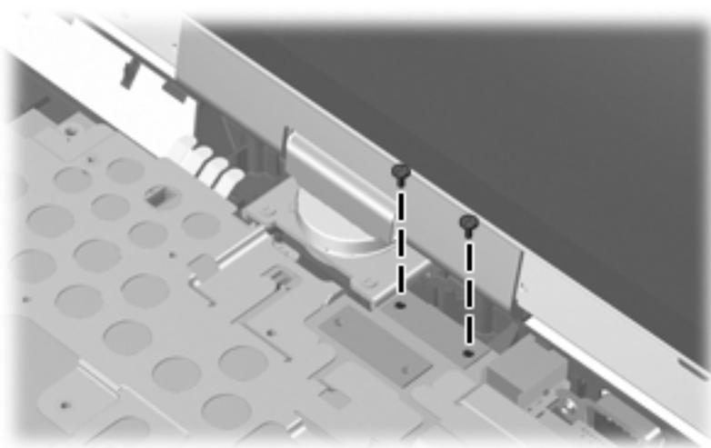
**Where used:** 2 screws that secure the display panel cable to the system board
