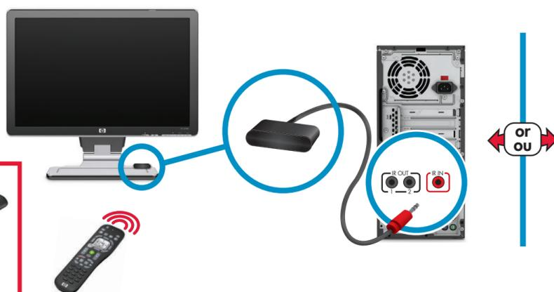
If you use a cable or satellite set-top box, pass the signal through the remote sensor control cable.
