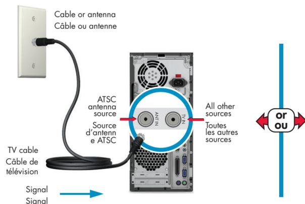
If you use a cable or satellite set-top box, pass the signal through the box.
