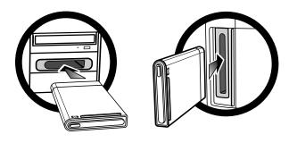
To insert the HP Pocket Media Drive into a specially designed HP computer:
