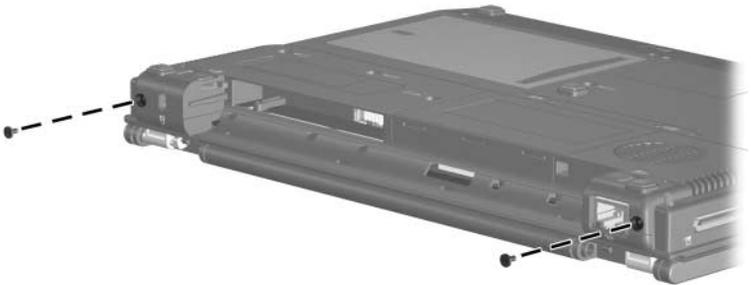
*Removing the Display Assembly Screws*
