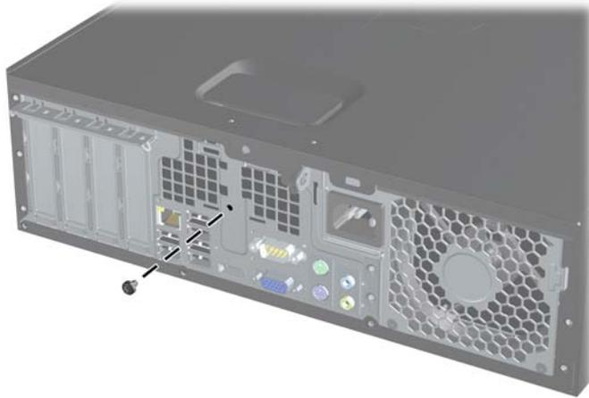
You can now remove the access panel. See [Removing the Computer Access Panel on page 4](#).
