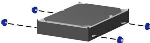
12. Align the guide screws with the slots on the chassis drive cage, press the hard drive down into the bay, then slide it back until it stops and locks in place.
