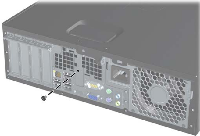
Gambar 1 Melepas Sekrup Smart Cover Lock
