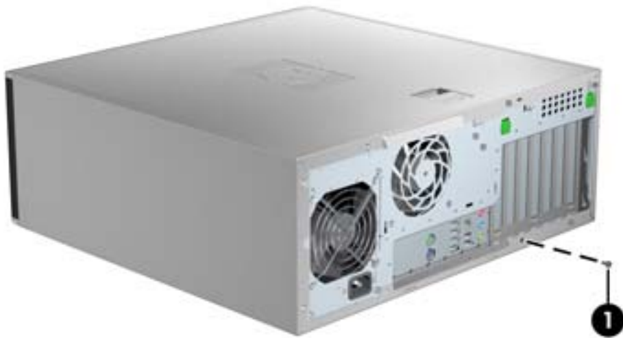
Figure 2 Removing the chassis screws
