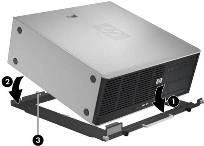
Figure 4 Installing the workstation on the tray
