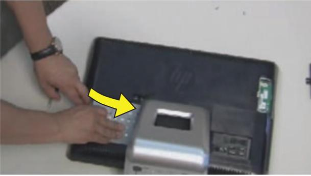
**3** Tighten the captive screw on the hard disk drive cage.
