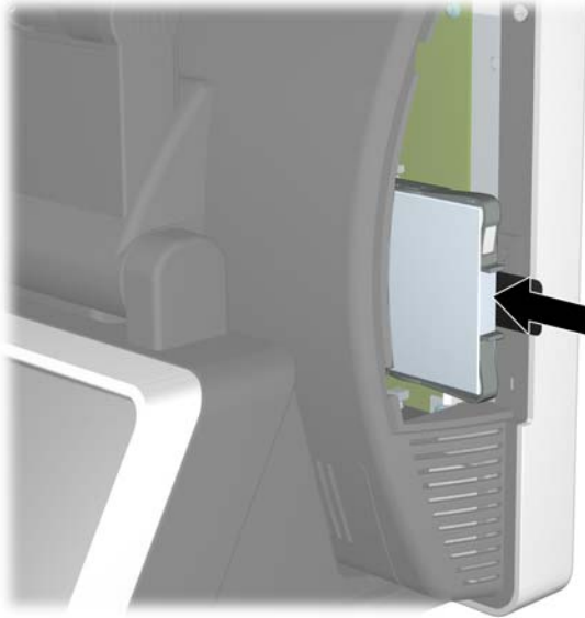
Figure 7-18 Replacing the Hard Drive
