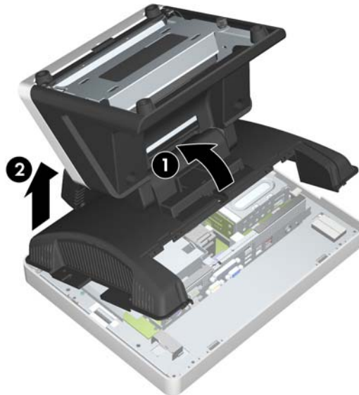
Figure 7-25 Removing the Display Head
