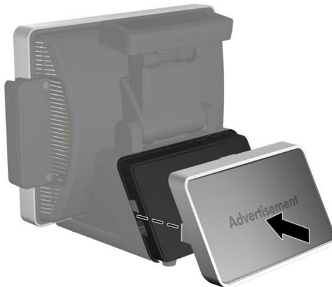
Figure 7-8 Replacing the Print Advertisement Panel Cover
