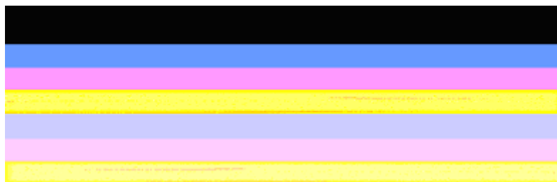
Example of Bad Color Bars: The yellow bar is streaked with another color.
