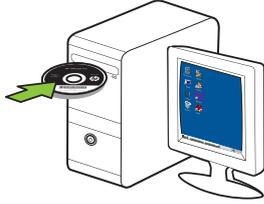
**EN** **Windows:** Install software first. Do NOT connect the USB cable until prompted.
