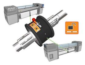
20. Go to the front panel and select the Substrate menu , then **Substrate management**, and press OK. Select **Carriage beam position** > **Move to printing (normal)** to lower the carriage beam into its normal position, close to the substrate. This process takes about 2 minutes to complete.
