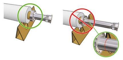
**10.** Ensure that the roll core fits tightly on the hub.
