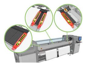
19. Unlock the differentials on the input and output spindles.
