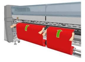
**14.** Install the two central edge holders, which can be done most easily at this stage.
