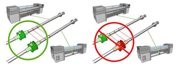
2. When both differential hubs are correctly positioned, use an Allen key 6 to tighten the screws and secure them in place. If a differential hub is loose, the substrate could become skewed during printing.
