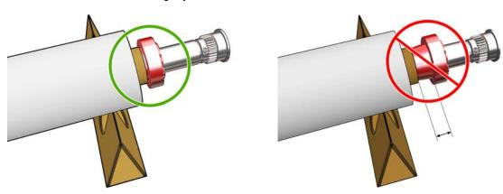
**11.** Ensure that the roll core fits tightly on the differential hub.
