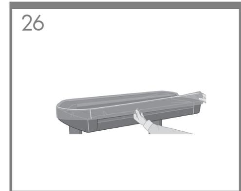
Keep out dust and reduce maintenance time: when not in use, cover your scanner with the plastic dust cover. **Caution:** make sure the scanner power is OFF when using the scanner dust cover.
