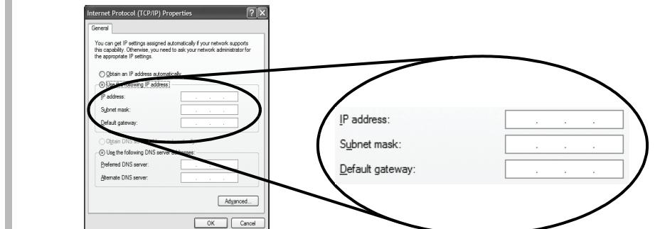
Enter the IP address, Subnet Mask and Default Gateway. Contact your IT Administrator or Internet Service Provider for details regarding IP address information. Record the IP address information for use in step B12.
