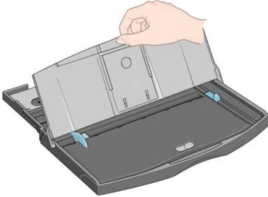
3. If the paper you are using is larger than Legal- or A4-size, move the small tab in the center towards the left so that you can lengthen the tray. Let go of the tab and pull the tray extension out as far as it will go.
