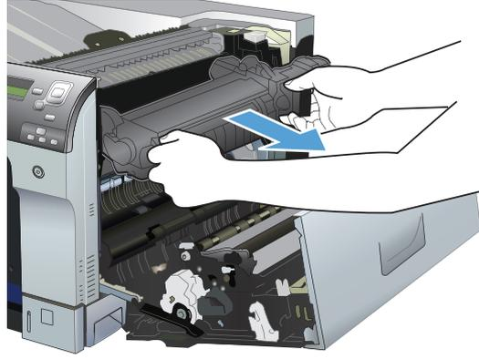
**EN** Pull the fuser straight out of the product to remove it.
