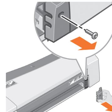
Remove the right plastic insert by extracting the screw as shown.
