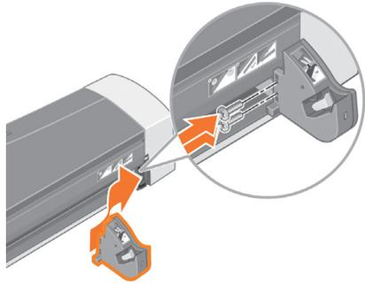
Install the right roll feed assembly, by aligning it with the guides and sliding it into position then using two screws to hold it in place. You may have a screw left over after assembly has been completed.
