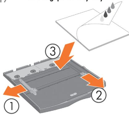
Place the sheets of paper into the corner of the input tray, print side facing down.
