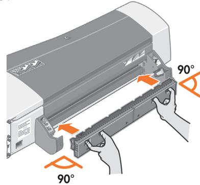
Insert the rear path until it clicks into place by pressing the buttons as shown, and carefully pushing it straight in.
