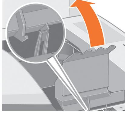
The hook at the front should unlatch itself. Lift the printhead cover back.
