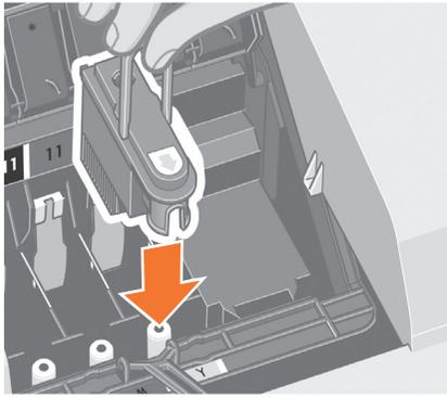
Match the color of the printhead to the slot in the printer.
