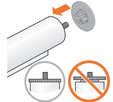
Insert the blue removable stop onto the spindle. Ensure it is correctly seated as shown above.
