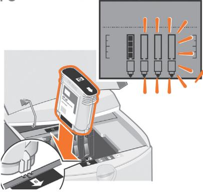
Match the color of the cartridge to the slot in the printer. As the ink cartridges are inserted the front panel will change.
