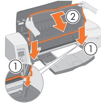
1. Lower the output tray into the printer vertically until it clicks into place and then 2. lower it onto the input tray, sliding the tray slightly to the left may help.
