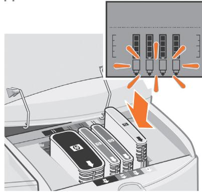
When the last ink cartridge is inserted only the printhead icons should be flashing.
