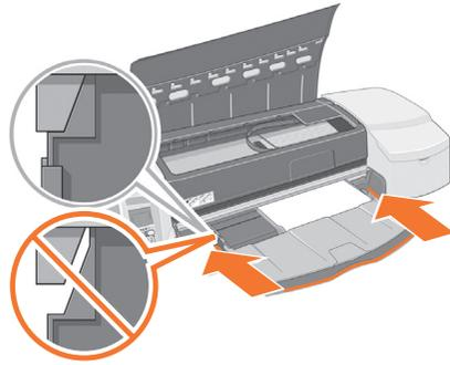
Insert the input tray as far as it will go into the printer, by pushing on both sides. Do not leave a gap between the tray and the printer.
