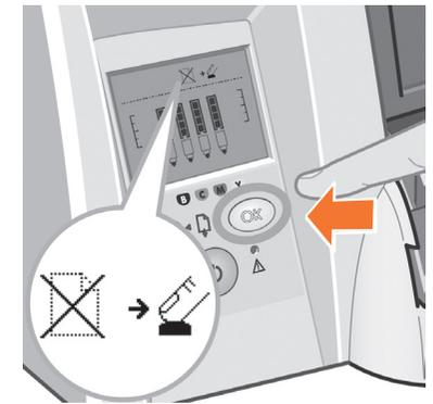
When the two above icons appear; load a single sheet into the front of the printer (see instructions on the printer's cover label), and press the OK Key, or load a roll. The printer will then automatically perform a printhead alignment, and a sheet will be ejected.
