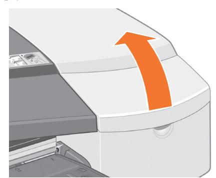
Open the first hinged flap at the right of the printer.
