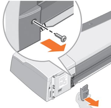
Remove the left plastic insert by extracting the screw as shown.
