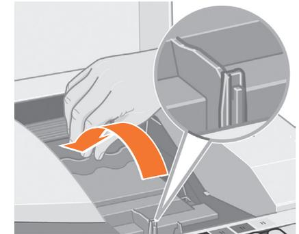
Return the printhead cover to its original position ensuring that the hook and the latch engage.
