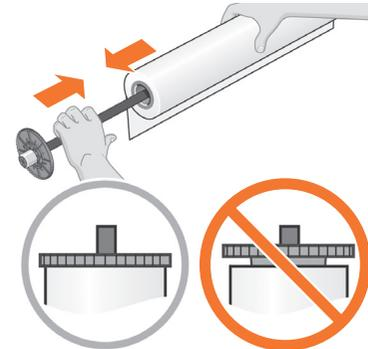
Insert the spindle into the roll taking care that the leading edge of the roll is on the correct side of the spindle. Ensure the roll is correctly seated as shown above.
