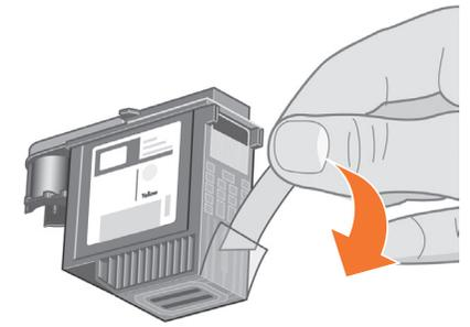
Unpack the printheads and remove the protective tapes.
