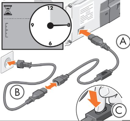
If a short power cable with a switch (A) has been supplied; connect it to the printer, and to the long power cable (B). Otherwise; connect the long cable to the printer (B). Connect the other end to a power socket. Wait 15 seconds. Press the switch (C).
