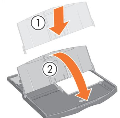
Locate the dust cover and insert it into the input tray from above and lower it down.
