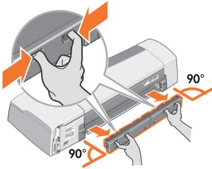
Remove the rear path by pressing the buttons as shown, and carefully pulling it straight out.
