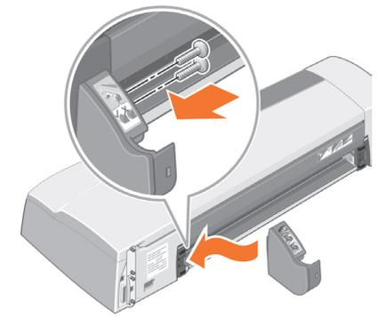
Install the left roll feed assembly, by aligning it with the guides and sliding it into position then using two screws to hold it in place.
