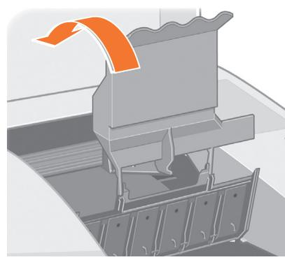
Lift the whole printhead cover back so that the printhead slots are exposed.
