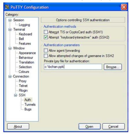
16. Enter the logon name associated with the public key. The public key in iLO 2 authenticates with the private key in PuTTY. If the keys match, you are logged into iLO 2 without using a password. Keys can be created with a key passphrase. If a key passphrase was used to generate the public key, you are prompted for the key passphrase before you log into iLO 2.
