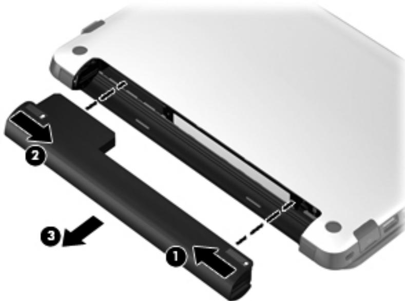
Reverse this procedure to install a battery.
