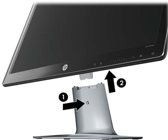
Gambar 2-1 Melepaskan Panel Monitor
