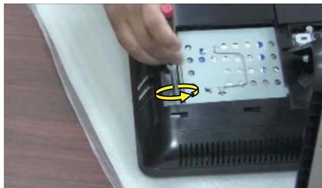
**3** Replace the four screws on the hard disk drive cage.
