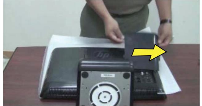
**IMPORTANT:** If you are removing both cards, you must remove the upper one before removing the lower one.
