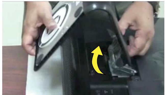
**11** Use a flathead screwdriver to remove the plastic tabs covering the two screw holes on the back cover.
