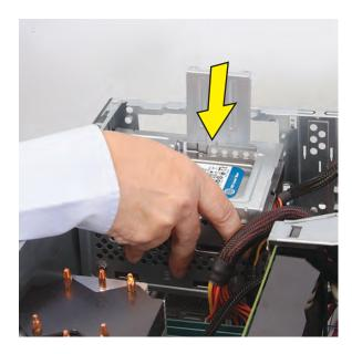
7 Slide the cage toward the bottom of the computer until it locks into place.
