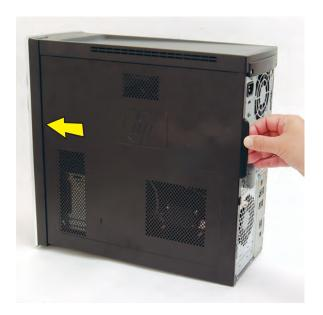
Tighten the side panel thumbscrew on the back of the computer.
