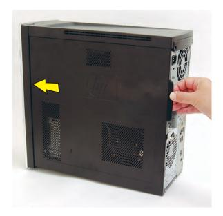
**18** Tighten the side panel thumbscrew on the back of the computer.
