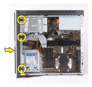
**12** Hold the side panel over the side of the computer with the front edge of the panel about 2.5 cm (1 inch) from the front of the computer.
