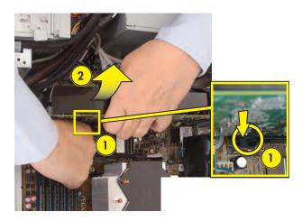
Move the card toward the inside of the computer to free the card external connectors from the computer slot, and then lift the card out of the computer.
