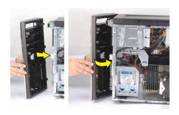
**11** Press the front panel into the computer.
