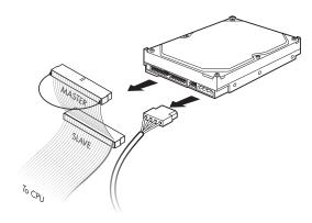
**16** Remove the four screws (two on each side) that secure the drive in the cage.
