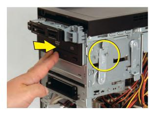
5 Hold the front panel over the computer, and then press the left side of the panel, inserting the tabs into the computer. Swing the right side of the panel toward the computer.
