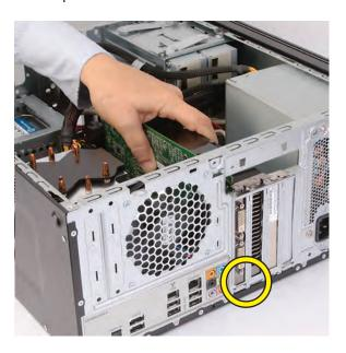
5 Press the card straight down until it is fully seated in the socket and fills the slots.
