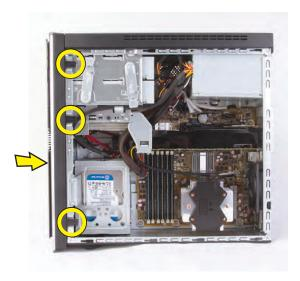
**3** Hold the side panel over the side of the computer with the front edge of the panel about 2.5 cm (1 inch) from the front of the computer.
