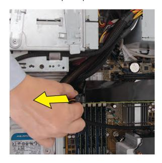
17 If present, disconnect any cables connected to a short or standard length card.
