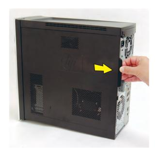
Tilt out the top of the side panel, and then lift the panel from the computer.
