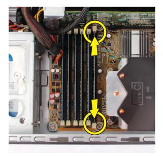
**10** Touching only the top edge of the memory module, lift it out of the socket.
