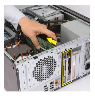
If there is no release latch, gently rock the card to free it, and then lift the card from the socket. Move the card toward the inside of the computer to free the card external connectors from the computer slot, and then lift the card out of the computer.
