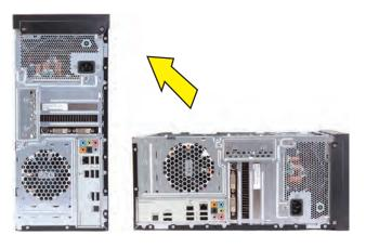
10 Hold the front panel over the computer, and then press the left side of the panel, inserting the tabs into the computer. Swing the right side of the panel toward the computer.
