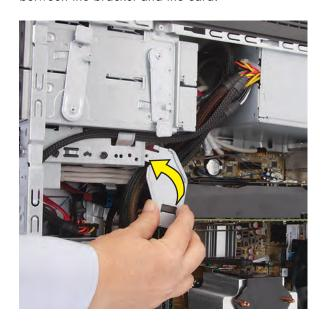
10 Insert and tighten the two screws that secure the inside bracket in the computer. Note that you need a flathead screwdriver with a long shaft to insert the lower screw.
