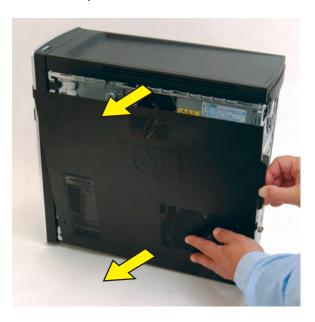
Locate the three tabs that secure the front panel to the computer. Pull each of the tabs out slightly, away from the computer, to release the panel.
