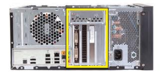
**9** On the back of the computer, remove the screw from the bracket cover for the add-in cards. If it is present, also remove the additional screw that secures a large graphics card.
