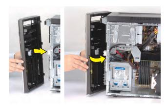
**6** Press the front panel into the computer.
