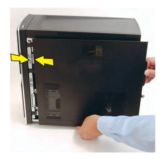
4 Place the bottom of the panel on the computer, inserting the tabs on the inside of the panel into the rail slots on the computer. Swing the top of the panel toward the computer, inserting the top tabs into the rail slots.
