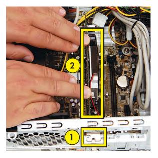
**2** Connect any cables to the card. Skip to step 11.
