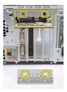
**12** Replace the bracket cover onto the back of the computer: Align the bracket cover hooks over the slots on the computer, and then...
