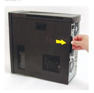
Tilt out the top of the side panel, and then lift the panel from the computer.
