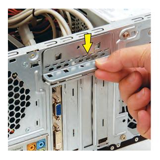
**13** Insert and tighten the bracket cover screw. If it is present, also insert and tighten the additional screw that secures a large graphics card.
