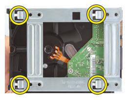
**4** Locate the four slots inside the computer that match the tabs on the bottom of the hard disk drive cage.
