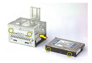
2 Insert and tighten the four screws that secure the drive in the cage.
