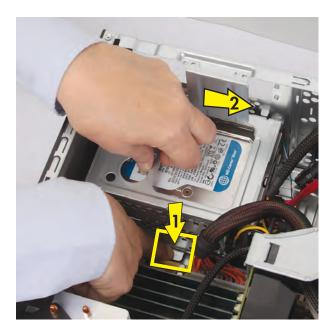
**14** Lift the cage partway out of the computer.
