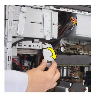
Pull the inside bracket from the computer. You may have to move cables out of the way as you withdraw the bracket.
