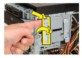
**4** Push the drive completely into the computer, until the drive latch locks it into place in the hole labeled 2 on the computer.
