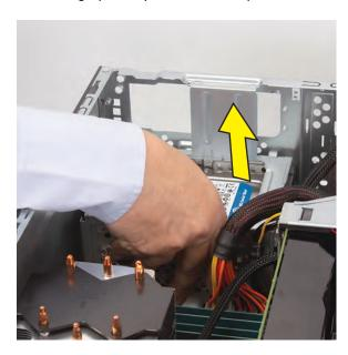
**15** Disconnect the cables from the hard disk drive in the cage:
