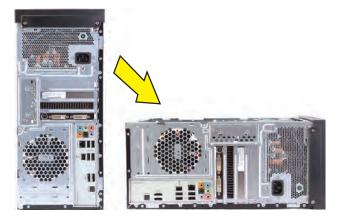
Locate the add-in cards on the back of the computer. Identify the one you want to replace.
