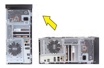
5 Hold the side panel over the side of the computer with the front edge of the panel about 2.5 cm (1 inch) from the front of the computer.
