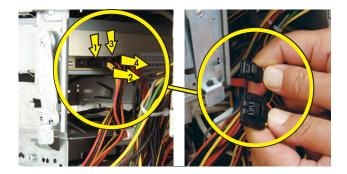
**14** Pull the drive completely out through the front of the computer.
