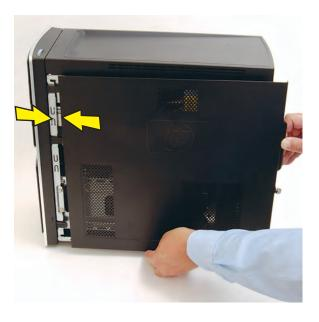
16 Place the bottom of the panel on the computer, inserting the tabs on the inside of the panel into the rail slots on the computer. Swing the top of the panel toward the computer, inserting the top tabs into the rail slots.
