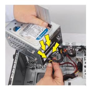
**6** Lower the cage into the computer, inserting the four tabs on the bottom of the cage into the computer slots.
