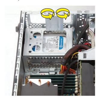
Locate the latch for the hard disk drive cage inside the computer.
