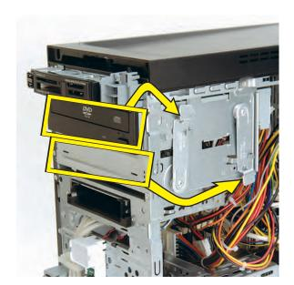
11 Pull out the drive latch (1), and then swing it to the left until it is in the center position (2).
