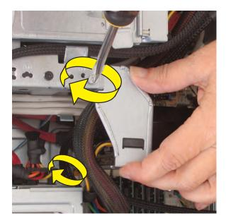
11 Look at the outside bracket cover for the two hooks that fit over the two slots on the back of the computer.
