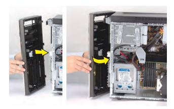
**2** Press the front panel into the computer.
