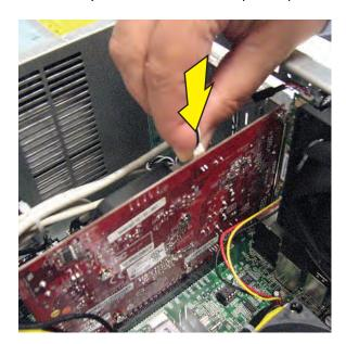
**3** For a long graphics card, lower the card into the computer, then move the card over the socket and toward the open slots.
