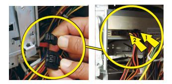
**3** Pull out the drive latch (1), swing it to the right (2), and release it into the hole labeled 2 on the computer.
