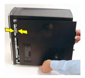
13 Place the bottom of the panel on the computer, inserting the tabs on the inside of the panel into the rail slots on the computer. Swing the top of the panel toward the computer, inserting the top tabs into the rail slots.
