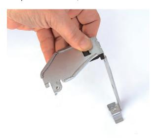
8 ...insert the inside bracket over the long graphics card placing the foot of the bracket over the lower screw hole in the computer. You may have to move cables out of the way as you insert the bracket.
