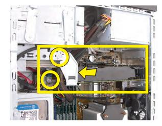
12 Remove the two screws that secure the inside bracket in the computer. You may have to move cabling out of the way to reach the lower screw. Note that you need a flathead screwdriver with a long shaft to remove the lower screw.
