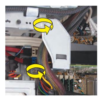
Twist the inside bracket clock-wise to free the top of the bracket from the drive cage.
