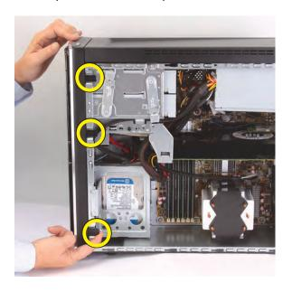
Swing the front panel open toward the left, and then lift it off the computer.
