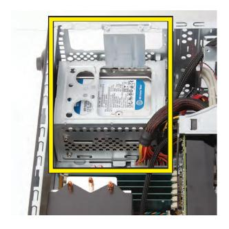
Remove the two screws that secure the drive cage in the computer.
