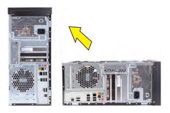
15 Hold the side panel over the side of the computer with the front edge of the panel about 2.5 cm (1 inch) from the front of the computer.
