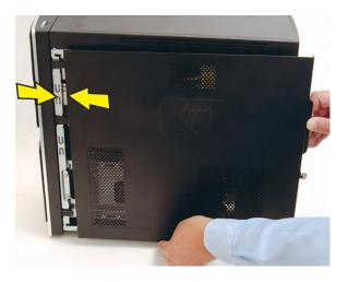
**8** Place the bottom of the panel on the computer, inserting the tabs on the inside of the panel into the rail slots on the computer. Swing the top of the panel toward the computer, inserting the top tabs into the rail slots.
