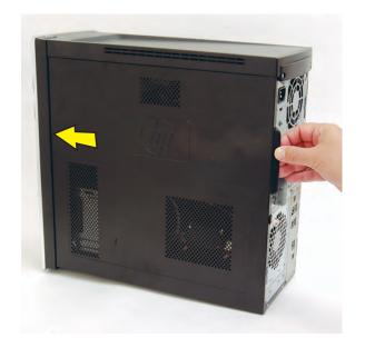
**6** Tighten the side panel thumbscrew on the back of the computer.
