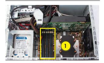
**9** Push down the retaining clip on each end of the memory socket to release the memory module.
