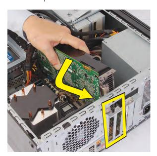
4 Place the foot of the card external end into the bottom of the open slots.
