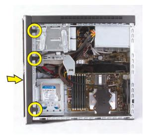
7 Hold the side panel over the side of the computer with the front edge of the panel about 2.5 cm (1 inch) from the front of the computer.
