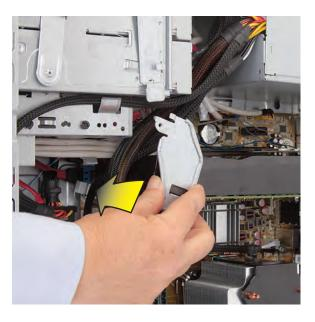
Twist the top of the inside bracket counter-clockwise into place over the graphics card power connector and into the drive cage. You may have to press the inside bracket down onto the graphics card and power connector as you twist it to insert the tip of the bracket into the drive cage. Ensure there is nothing between the bracket and the card.
