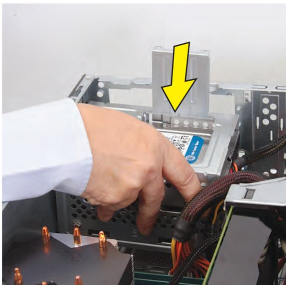
**8** Insert and tighten the two screws that secure the cage in the computer.
