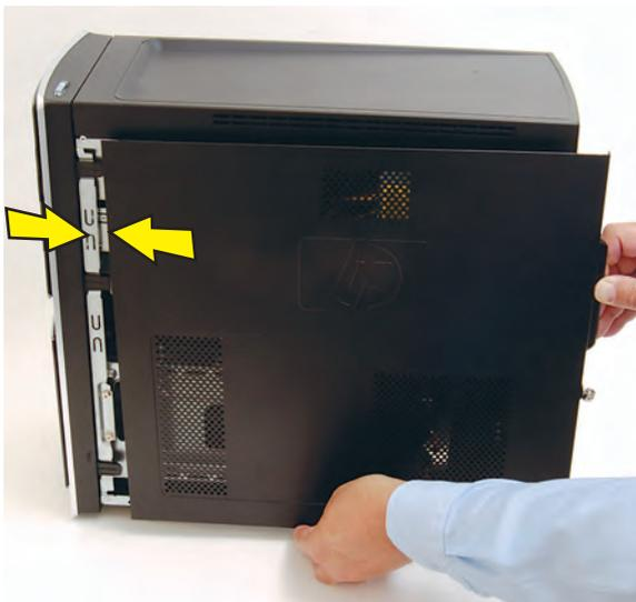
**13** Place the bottom of the panel on the computer, inserting the tabs on the inside of the panel into the rail slots on the computer. Swing the top of the panel toward the computer, inserting the top tabs into the rail slots.
