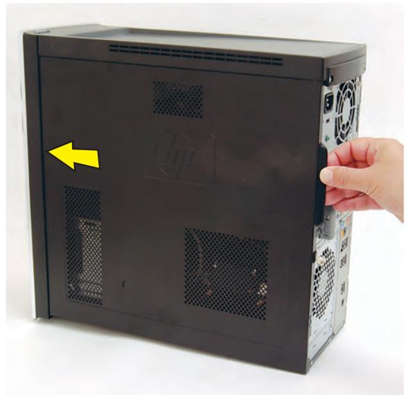
**8** Tighten the side panel thumbscrew on the back of the computer.
