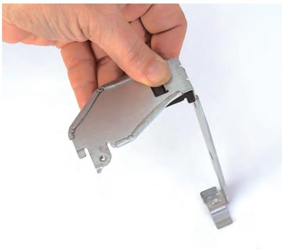
9 Twist the top of the inside bracket counter-clockwise into place over the graphics card power connector and into the drive cage. You may have to press the inside bracket down onto the graphics card and power connector as you twist it to insert the tip of the bracket into the drive cage. Ensure there is nothing between the bracket and the card.
