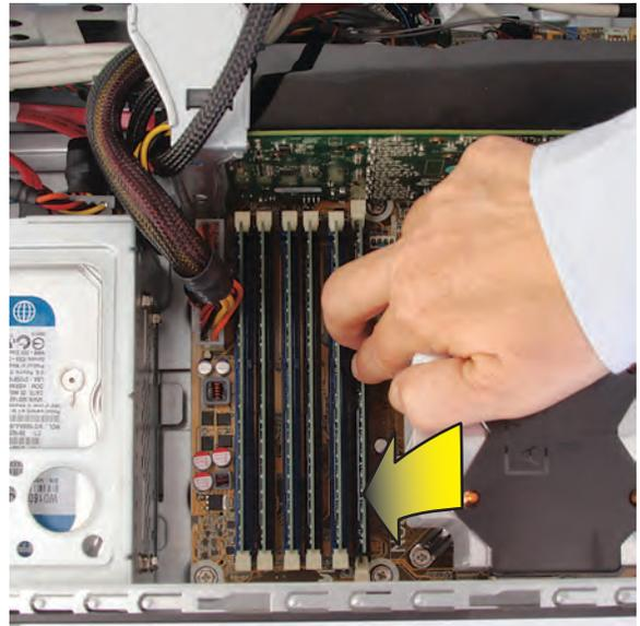
...until the retaining clips at the ends of the socket lock the module into place.
