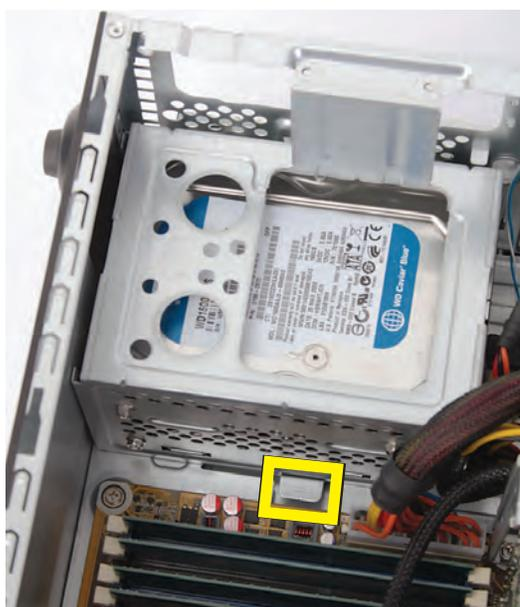
**13** Press the cage latch (**1**), and slide the hard disk drive cage toward the top of the computer (**2**) to release it.
