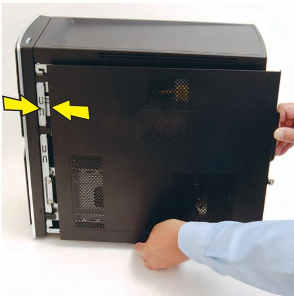
**6** Place the bottom of the panel on the computer, inserting the tabs on the inside of the panel into the rail slots on the computer. Swing the top of the panel toward the computer, inserting the top tabs into the rail slots.
