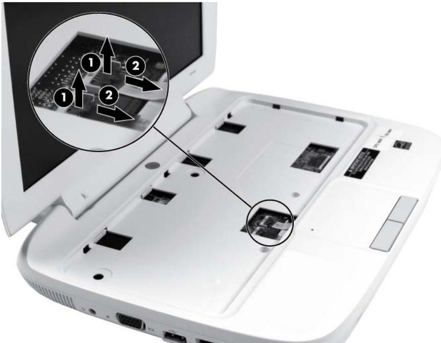
7. Remove the 2 Phillips PM2.0x5.5 screws (1) that secure the top cover to the base enclosure.
