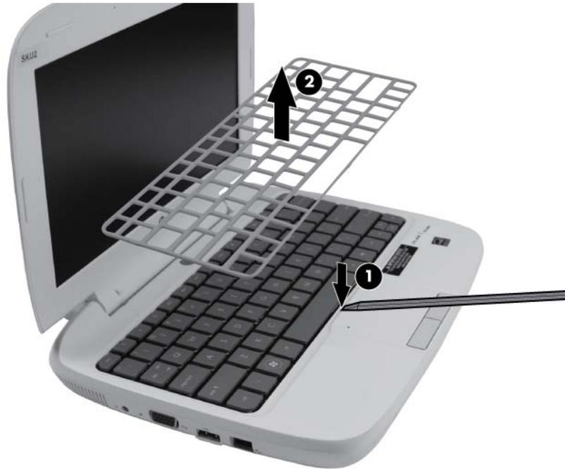
5. Lift up on the top edge of the keyboard and hold it at an angle.
