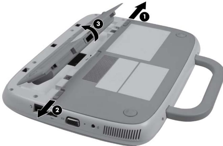
Reverse this procedure to install the battery.
