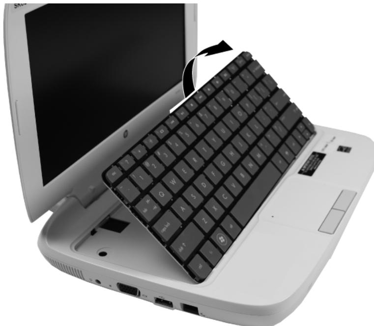
6. Release the zero insertion force (ZIF) connector (1) to which the keyboard cable is attached.
