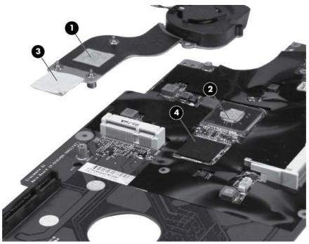
Reverse this procedure to install the fan and heat sink assembly.
