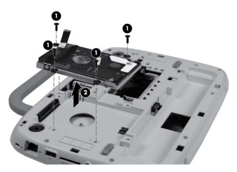
If it is necessary to replace the hard drive bracket, follow these steps:
