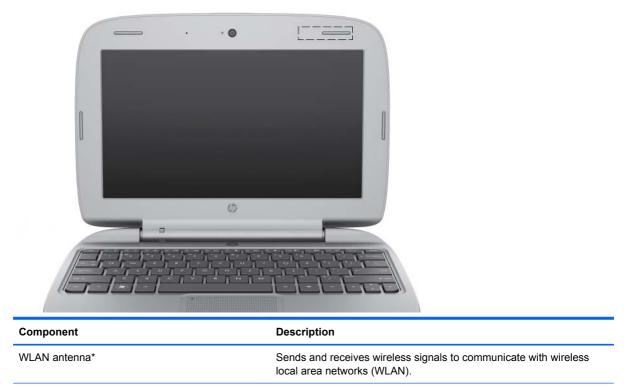
\*The antenna is not visible from the outside of the computer. For optimal transmission, keep the areas immediately around the antenna free from obstructions. To see wireless regulatory notices, refer to the section of the *Regulatory, Safety, and Environmental Notices* that applies to your country or region.
