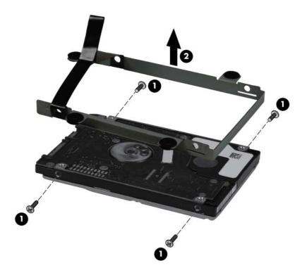
If it is necessary to replace the hard drive bracket grommets, remove the grommets from the hard drive bracket.
