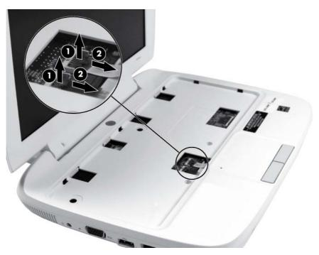
7. Remove the 2 Phillips PM2.0×5.5 screws (1) that secure the top cover to the base enclosure.
