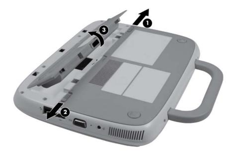
Reverse this procedure to install the battery.
