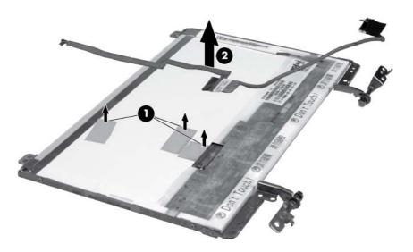
12. If it is necessary to replace the wireless antenna transceiver and cable, detach the cable from the adhesive (1) that secures it to the display back cover, and then remove the cable (2).
