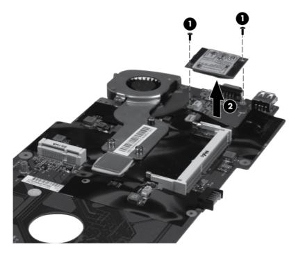
Reverse this procedure to install the modem.
