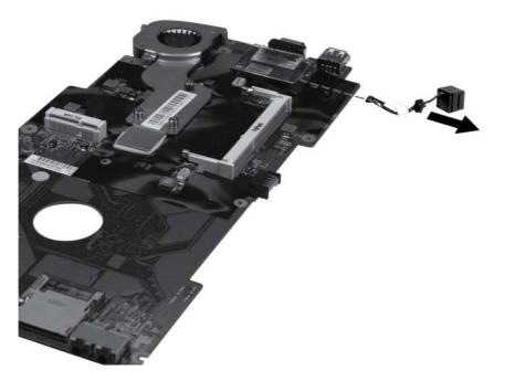
2. Remove the 2 Phillips 2.0×3.0 screws (1) that secure the modem to the system board.
