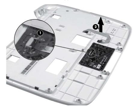
If it is necessary to replace the security cable slot bracket, follow these steps:
