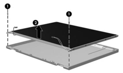
6. Remove the display panel assembly (2) from the display back cover.
