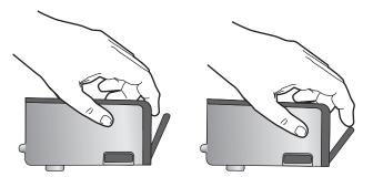
Reinstall the ink cartridge.It should now snap down into place.
