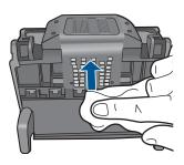
**b**. Use a fresh, lightly dampened, lint-free cloth to wipe any accumulated ink and debris from the edge between the nozzles and the contacts.
