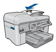
Slide paper-width guide inward until it stops at edge of paper.
