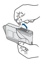
**b**. Twist orange cap to snap it off. A forceful twist may be required to remove the cap.
