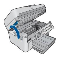
Remove every ink cartridge by pushing the tab on the ink cartridge and then pulling the ink cartridge out of its slot. Place the ink cartridges on a piece of paper with the ink openings pointing up.
