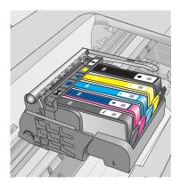
Printing cannot occur without one of each type of ink cartridge inserted into the correct slot.
