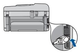
3. Connect the other end of the Ethernet cable to an available port on your Ethernet router, switch, or wireless router.
