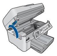
3. Remove all of the ink cartridges and place them on a piece of paper with the ink opening pointing up.
