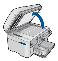
Load original print side down on right front corner of glass.
