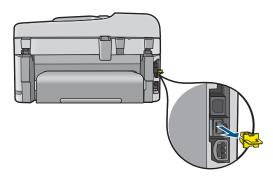
2. Connect the Ethernet cable to the Ethernet port on the back of the product.
