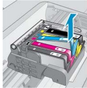
4. Lift the latch handle on the print carriage until it stops.
