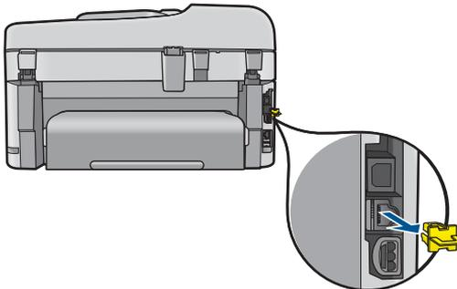
2. Connect the Ethernet cable to the Ethernet port on the back of the product.
