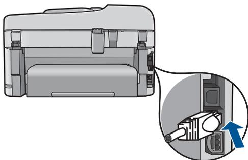
3. Connect the other end of the Ethernet cable to an available port on your Ethernet router, switch, or wireless router.
