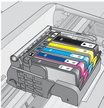
4. Run your finger along the top of the ink cartridges to locate any cartridges that are not snapped completely down.
