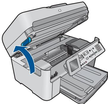
3. Remove every ink cartridge by pushing the tab on the ink cartridge and then pulling the ink cartridge out of its slot. Place the ink cartridges on a piece of paper with the ink openings pointing up.
