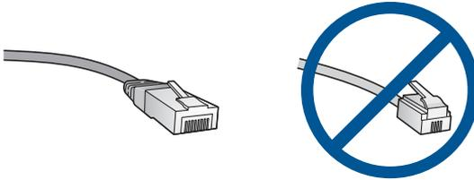
Although standard Ethernet cables look similar to standard telephone cables, they are not interchangeable. There is a different number of wires in each one, and each has a different connector. An Ethernet cable connector (also called an RJ-45 connector) is wider and thicker and always has 8 contacts on the end. A phone connector has between 2 and 6 contacts.
