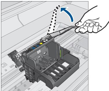
5. Remove the printhead by lifting it straight up.
