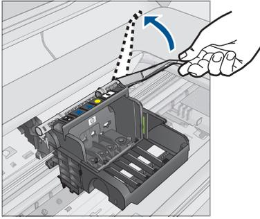
5. Remove the printhead by lifting it straight up.
