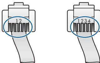
Make sure you used the phone cord supplied in the box with the product to connect to the telephone wall jack.
