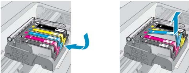
4. Lift the latch handle on the print carriage until it stops.
