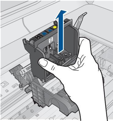
6. Make sure the latch handle is raised, and then reinsert the printhead.
