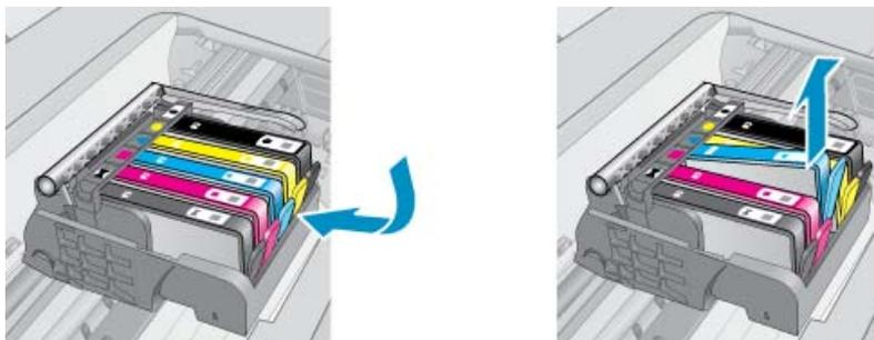
8. Press the ink cartridge back down into place. The tab should make a snapping noise when the ink cartridge is correctly seated. If the ink cartridge did not make a snapping noise, the tab might need to be readjusted.
