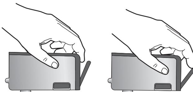
11. Reinstall the ink cartridge. It should now snap down into place.
