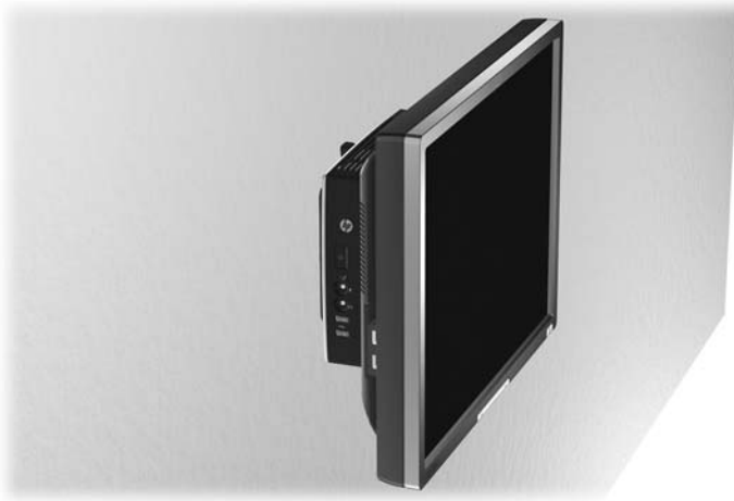
Figure C-6 Thin client mounted on back of monitor stand
