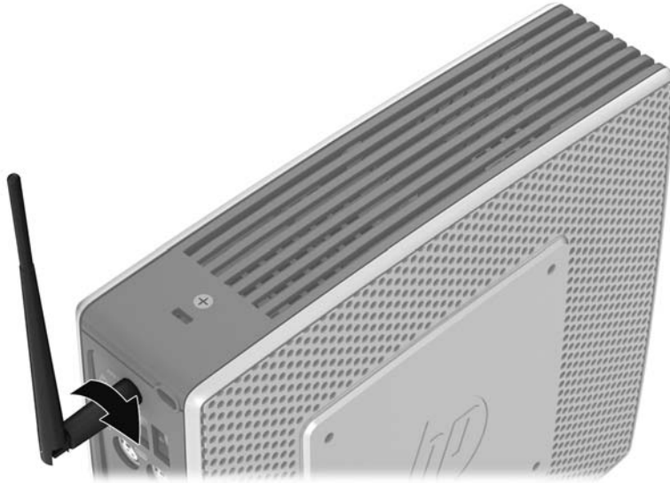
Figure 1-5 Installing the antenna
