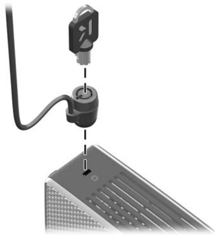
Figure B-1 Securing the thin client
