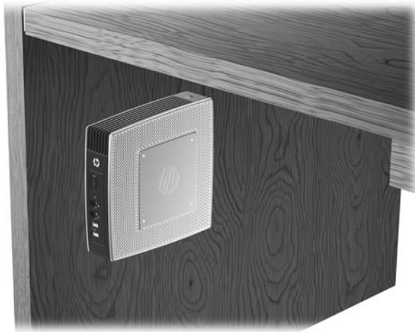
Figure C-8 Thin client mounted under desk
