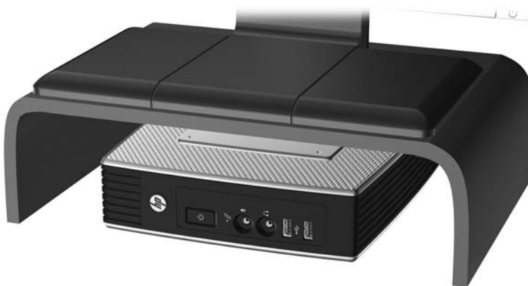
Figure D-3 Under monitor stand with at least one inch clearance
