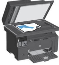
**EN Test copy.** Load the control-panel description page on the scanner glass, and then press the Start Copy
