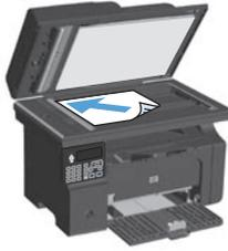
**EN** **Test scan.** Load the control-panel description page on the scanner glass. **Windows:** In the HP program group, select **Scan to**, and select a scanning destination. **Mac:** Open the HP Director, click **Scan**, and click **Scan** again. Click **Finish**, and then click **Destinations**. Name the file and specify the destination location. Click **Save**.
