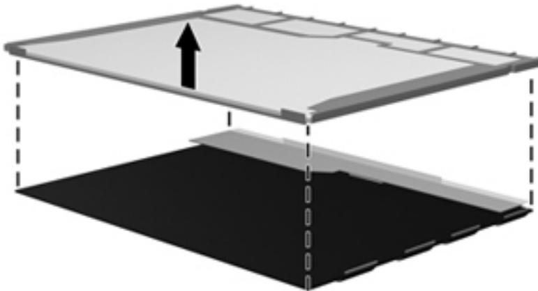
**24.** Recycle the LCD panel and backlight.
