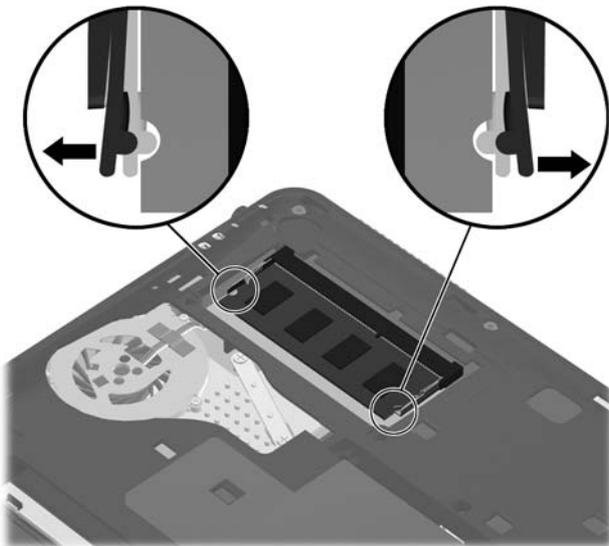
4. Remove the memory expansion module from the computer.
