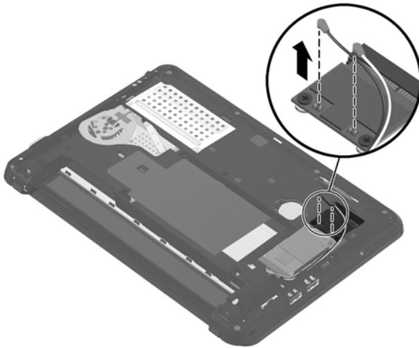
**NOTE:** The number of WLAN cables varies, depending on model. Note the labeling and position of the cables. Disconnect the antenna cables by pulling the cables off the terminals.
