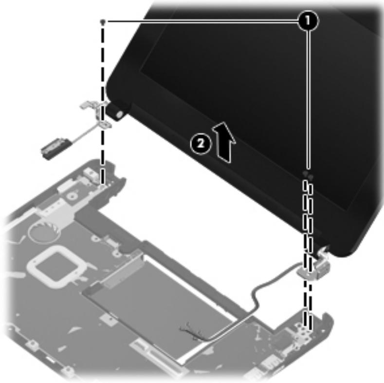
Reverse this procedure to reassemble and install the display assembly.
