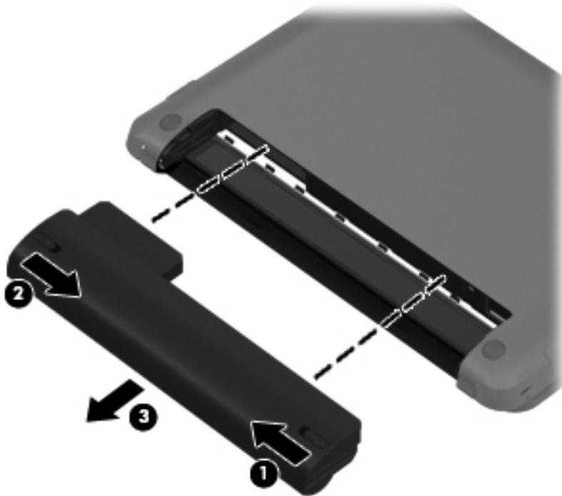
Reverse this procedure to install a battery.
