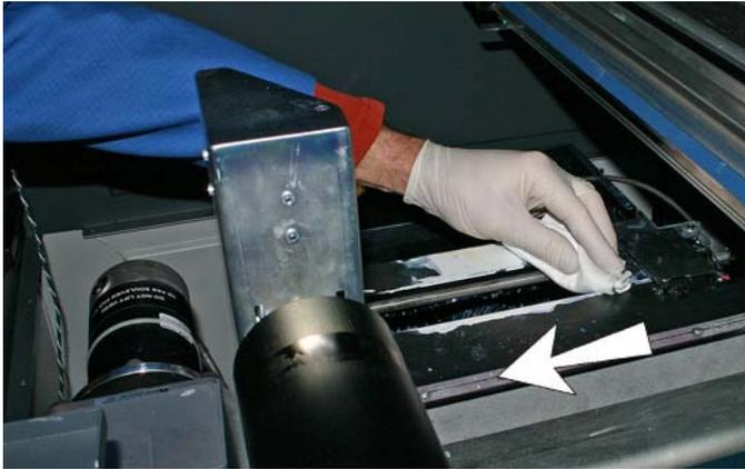
5. Using a lint-free cloth, clean both of the wiper rails on both sides of the wiper carriage. Clean the exposed rails on all sides, moving the wiper carriage to clean the full length of the rails.
