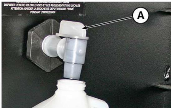
△ **CAUTION:** The drain spigot must remain closed during printing and service station use. An open spigot affects the vacuum level in the service station and will degrade service station performance if left open.
