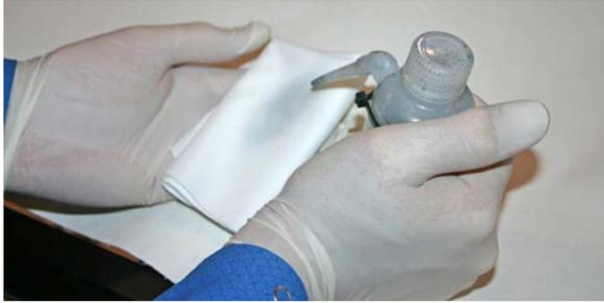
5. For each printhead, press a clean portion of the cloth with two fingers, each on one printhead, and draw the cloth across the printhead toward you (see A in the following figure).
