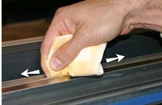
6. Using a lint-free cloth and Printhead Flush, clean the lower carriage-wheel strip from end to end on the rail (moving the carriage to clean the full length of the rail).
