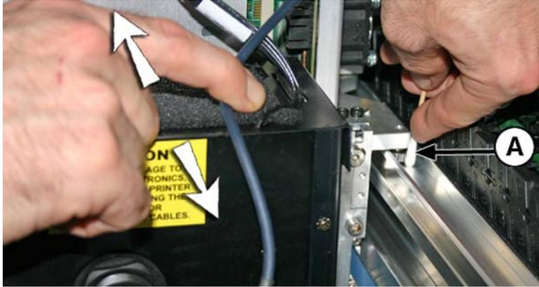
5. Clean the top slanted wheels by inserting an IPA moistened cotton swab into the opening above the wheels (A) and moving the carriage back and forth.
