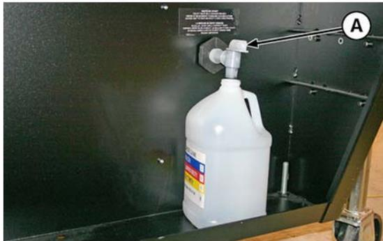
5. After the waste ink has drained, turn the spigot to the closed position
