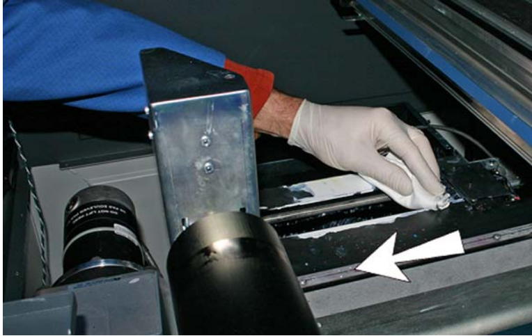
Figure 18 Cleaning the top of the service station
