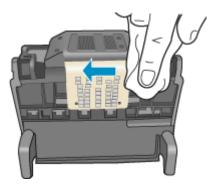
**c**. Use a fresh, lightly dampened, lint-free cloth to wipe the plastic ramps on both sides of the nozzles. Wipe away from the nozzles.
