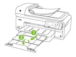
**NOTE:** When printing documents larger than A3/11 x 17 inches, extend the output tray extender all the way and tilt the paper stopper.
