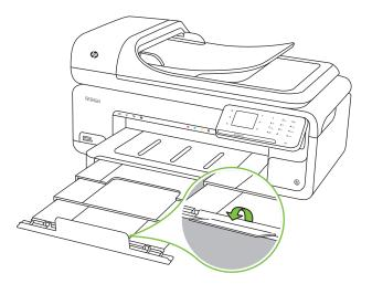
• Remove excess media from the output tray. There is a limit to the number of sheets the tray can hold.
