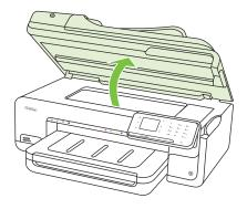
**3.** Remove all of the ink cartridges and place them on a piece of paper with the ink opening pointing up.
