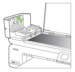
4. Lift the automatic document feeder mechanism.
