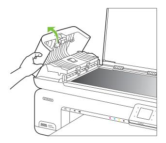
3. Continue lifting the automatic document feeder cover to the vertical position.
