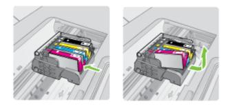
**4.** Lift the latch handle on the print carriage.
