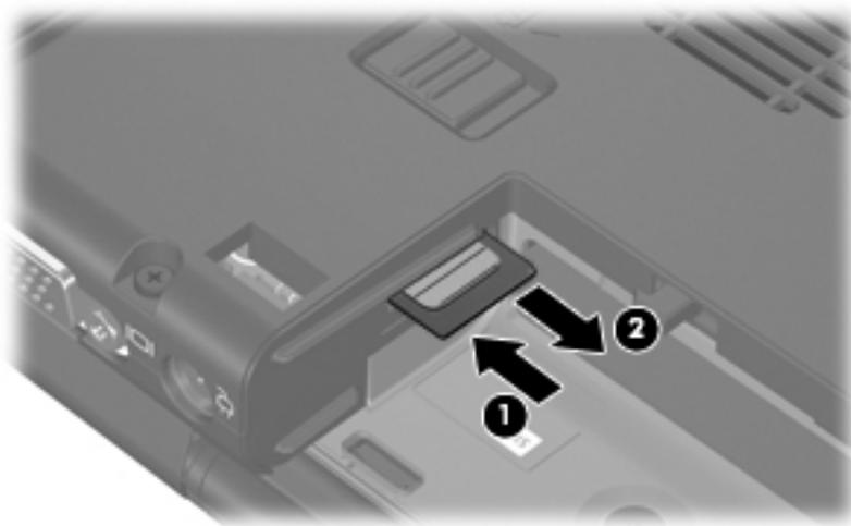
Reverse this procedure to install the SIM.
