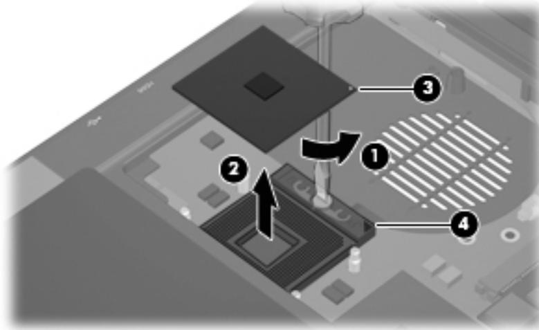
Reverse this procedure to install the processor.
