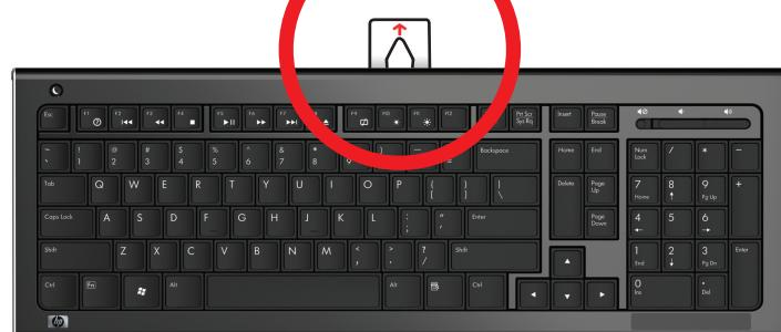
Pull tabs on the back of the keyboard and mouse to activate pre-installed batteries. Ensure the mouse power switch is in the "On" position. The keyboard and mouse are pre-synchronized for your convenience.
